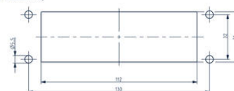
Panel cut-out for wall thickness 1.5 - 2 mm (for snap-on attachment)
