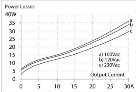
Fig. 9-2 Losses vs. output current at 12V, typ.
